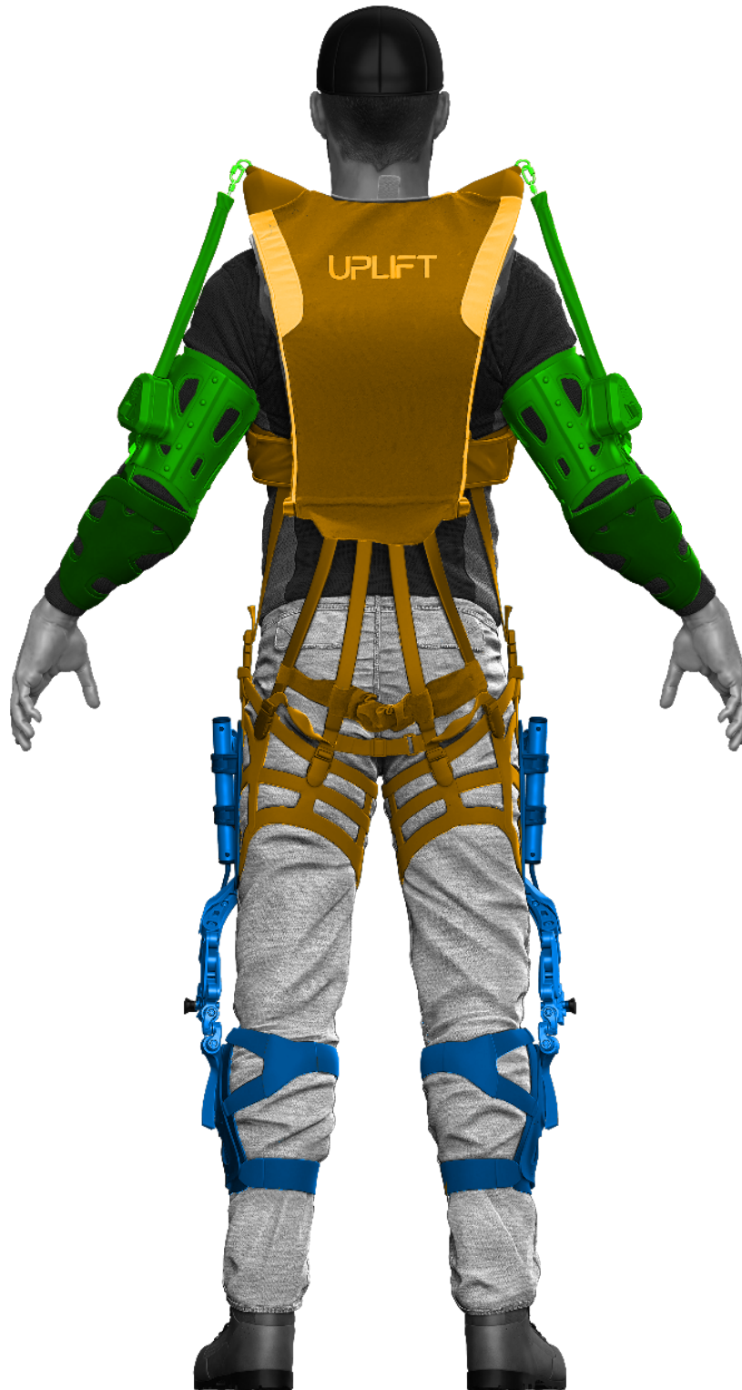
Figure 2 - In yellow: UPLIFT™ Back Module In green: UPLIFT™ Arm Module In blue: UPLIFT™ Leg Module
